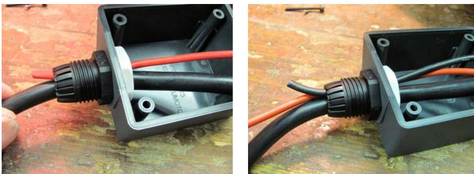
Figure 11. Thread red and black 12" cords through junction box hole.
