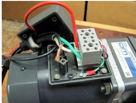
Figure 14. Connect green wire to  $\perp$  and the white wire to U1.
