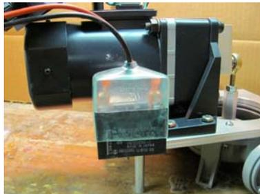
Figure 22. Install capacitor cap.
