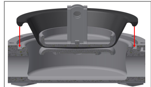
Outer lip of diaphragm fits into groove on pump body.
