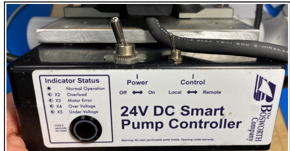
Pump Control box showing manual and remote activation switches and fault status indicator Figure 8
