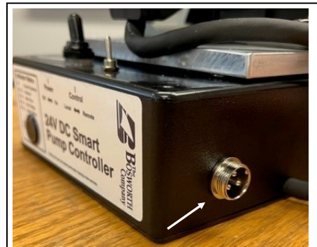
Remote Control Interface on side of Controller Box Figure 7
