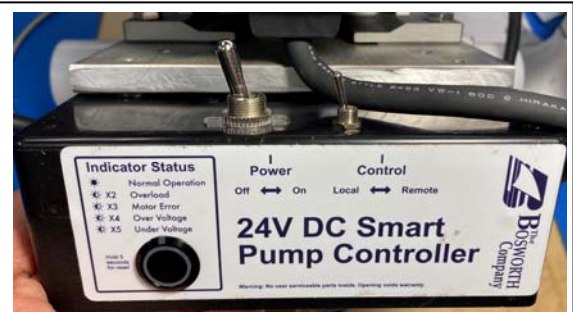
Pump Control box showing fault status indicator/reset button on left. Figure 2
