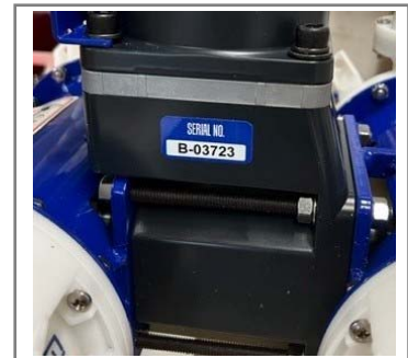
Pump serial number on side of motor Figure 1
