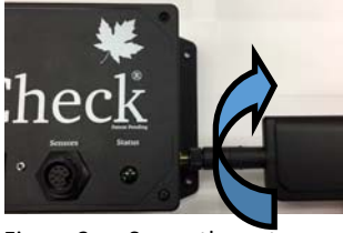
Figure 2a. Screw the antenna into the antenna port on the side of the SapCheck Controller.
