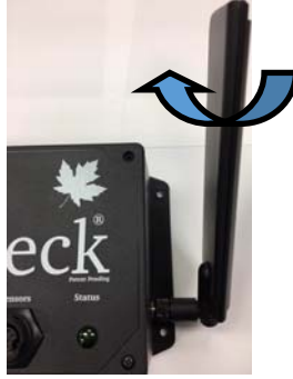
Figure 2b. Flip the antenna up. Optionally, rotate the antenna so that the flat side faces forward.
